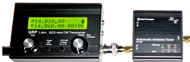
Example of using Automatic Antenna Tuner (KT-005) with QCX-mini transceiver
