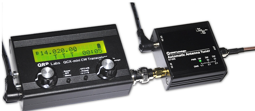
FIGURE 22. QCX-mini® and ATU (KT-005A) size comparison with BNC(m) to SMA(m) adapter (KT-005R) and power cord (KT-005C)
