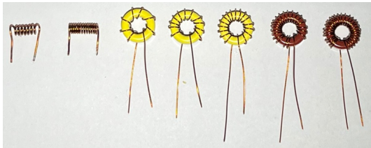
FIGURE 14. Coils ready to be mounted on the board (from left: L1 to L7)
