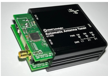
FIGURE 21. KT-005 just before closing the housing
